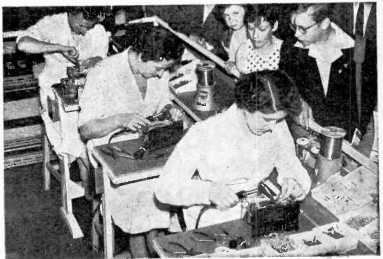
Left: Special camera used for electronic timing of Fairey Delta II aircraft. Right: Midget receivers being soldered with Multicore "Savbit" alloy containing copper to reduce bit wear.
